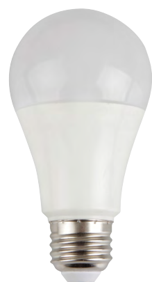
LED A19 / 10W / 120V 15,000Hrs / 80CRI / Non-Dimmable L7591-3 (2,700K / 800Lm) L7593-3 (3,000K / 830Lm) L7594-3 (4,000K / 840Lm) L7595-4 (5,000K / 800Lm)
