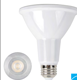
LED PAR30 / 12W / 850Lm / 120V 25,000Hrs / 90CRI / Dimmable L7531-3 (3,000K)
