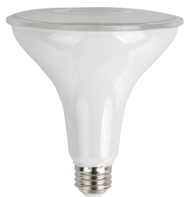
LED PAR38 / 12W / 1,050Lm / 120V 25,000Hrs / 90CRI / Dimmable L7532-3 (3,000K)
